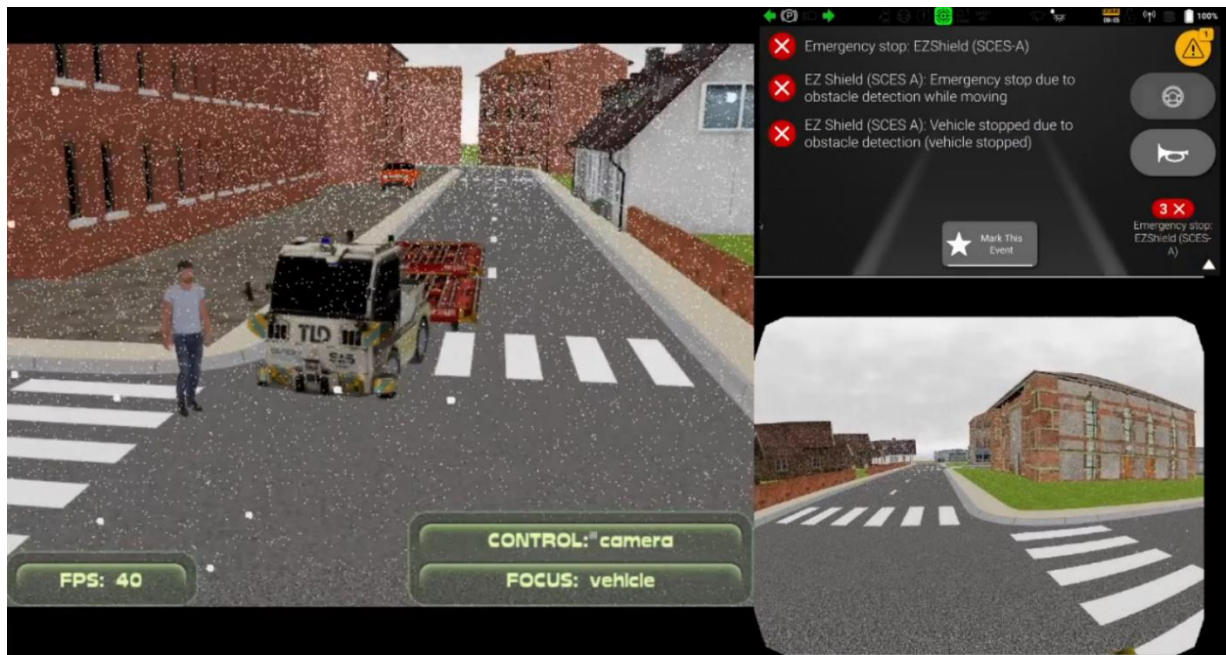
Figure 12. EZTow - Turn right, simulation in 100mm rain with a fully loaded trailer.
